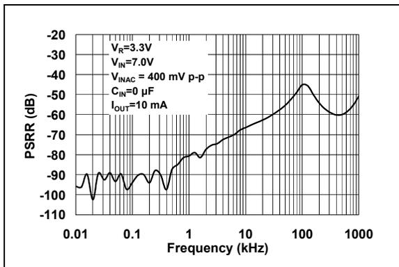
**FIGURE 2-15:** Power Supply Ripple Rejection vs. Frequency.
