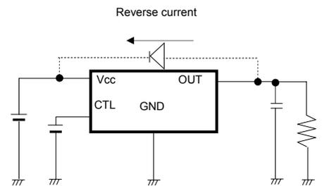
Fig.34: Bypass diode
