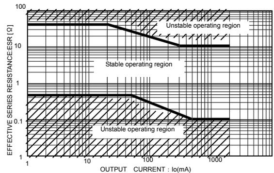
Fig.33: Io vs. ESR characteristics (BA00DD0)
