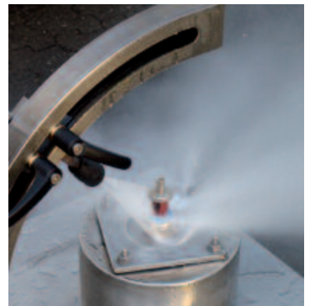
Fig. 6 PFLITSCH testing laboratory: Test IP69K
