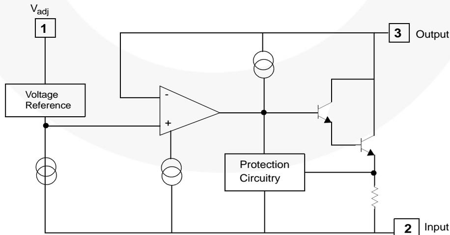
Figure 1. Block Diagram
