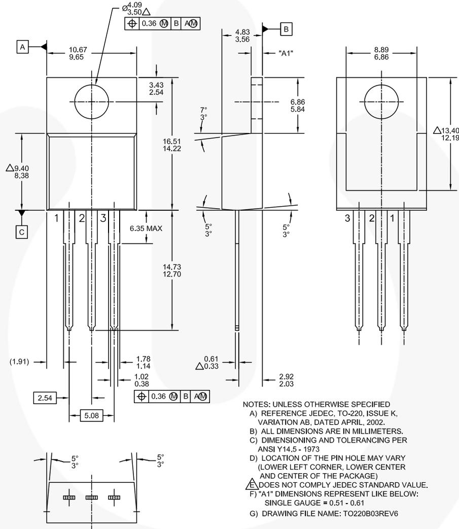
Figure 13. TO220, MOLDED, 3-LEAD, JEDEC, VARIATION AB
