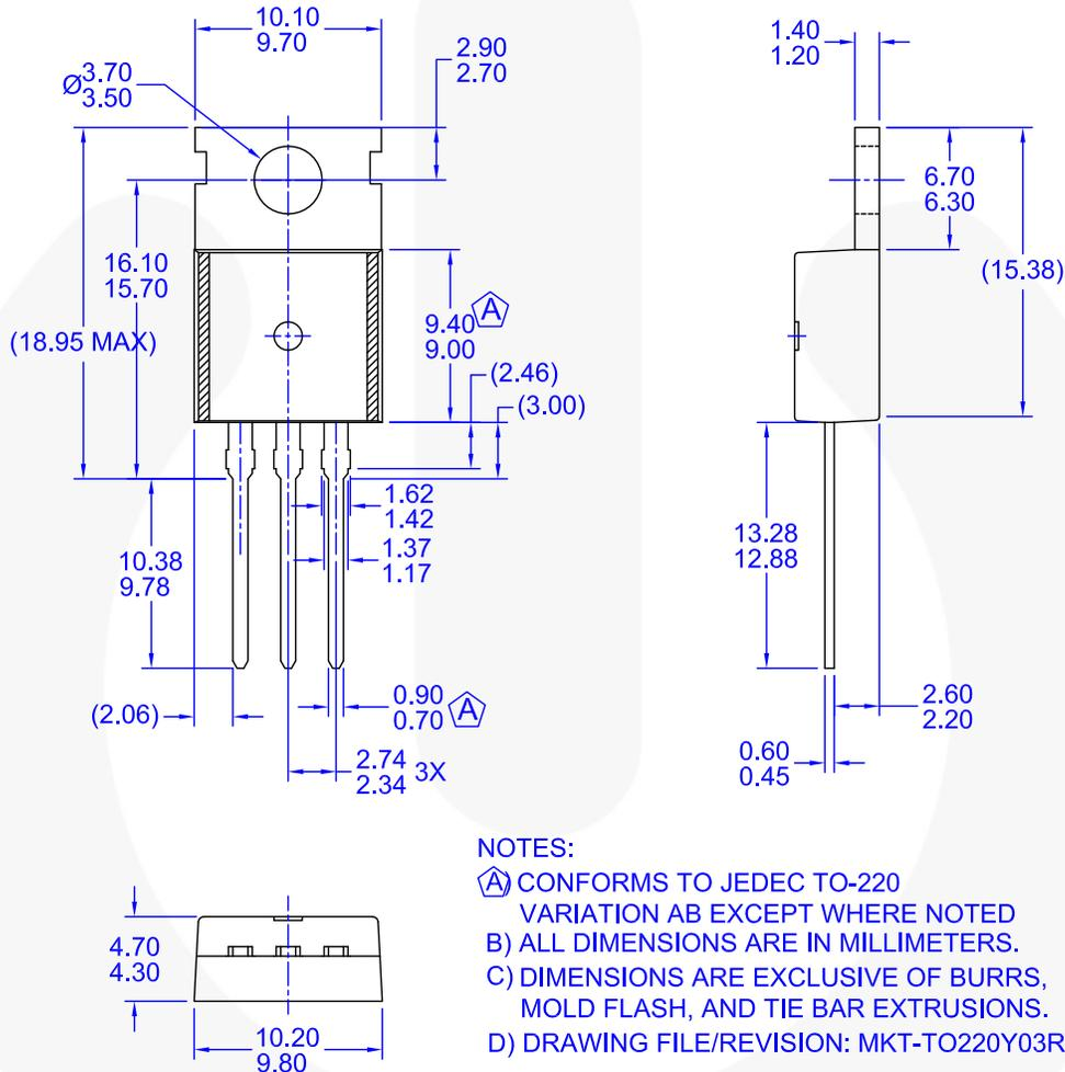
**Figure 14. TO220, MOLDED, 3-LEAD, NON-JEDEC, VARIATION AB**
