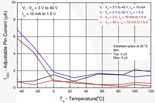
Figure 5. Adjustable Pin Current Change vs. Temperature
