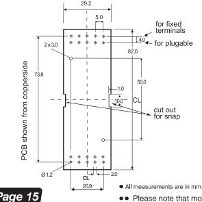
Module enclosure for M36 DIN-rail. Series 350 is, if requested, available in several colours and with customer specified holes in the front. Lid, PCB, customized label and packing is available.
