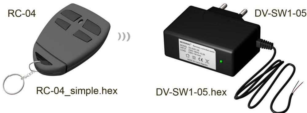
The TR module should be uploaded out of the DV-SW1-05 case in an external programmer. Wireless upload (RFPGM) is also possible. To enable this, the user must ensure a way to switch the TR in RFPGM mode, e.g. by the `enableRFPGM()` function (the TR is delivered with this option disabled).
