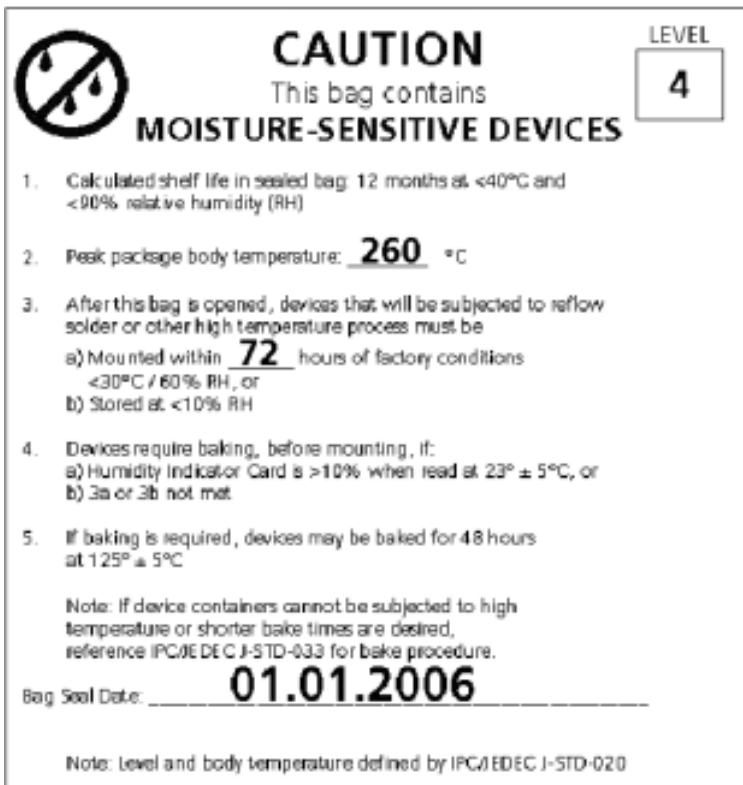
Figure 100: Applicable MSD Label (See Section 3.1 for baking instructions)
