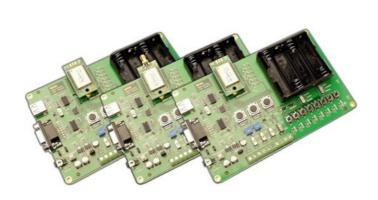
The **ProBee-ZE20SK** is the development kit for the ProBee-ZE2OS OEM module series. The ZE20-SK01 includes 3 development boards, antennas, cables, power supply, accessories, and CD with software and documentation.
