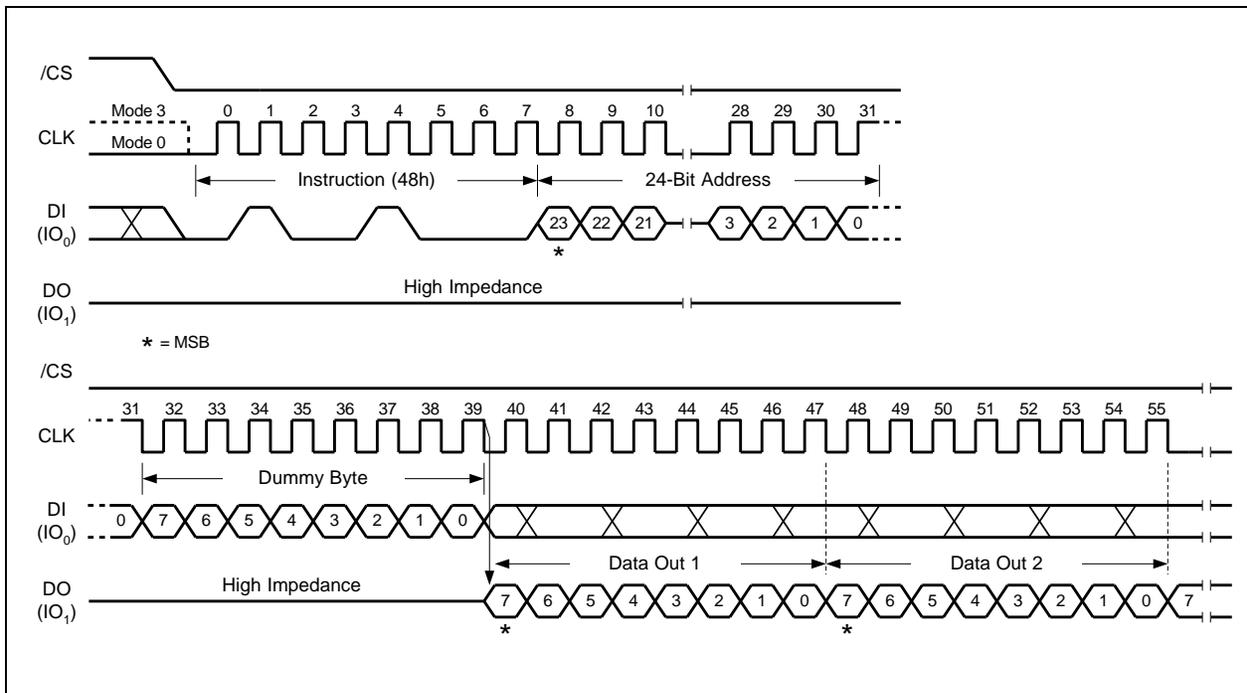
Figure 37. Read Security Registers Instruction (SPI Mode only)
