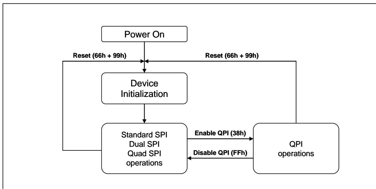
Figure 3. W25Q64FV Serial Flash Memory Operation Diagram
