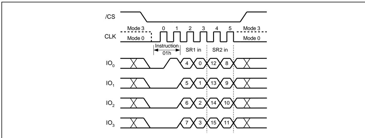
Figure 9b. Write Status Register Instruction (QPI Mode)
