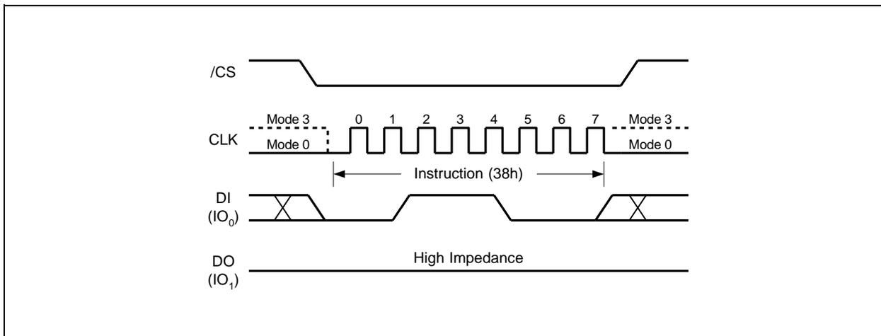
Figure 40. Enable QPI Instruction (SPI Mode only)
