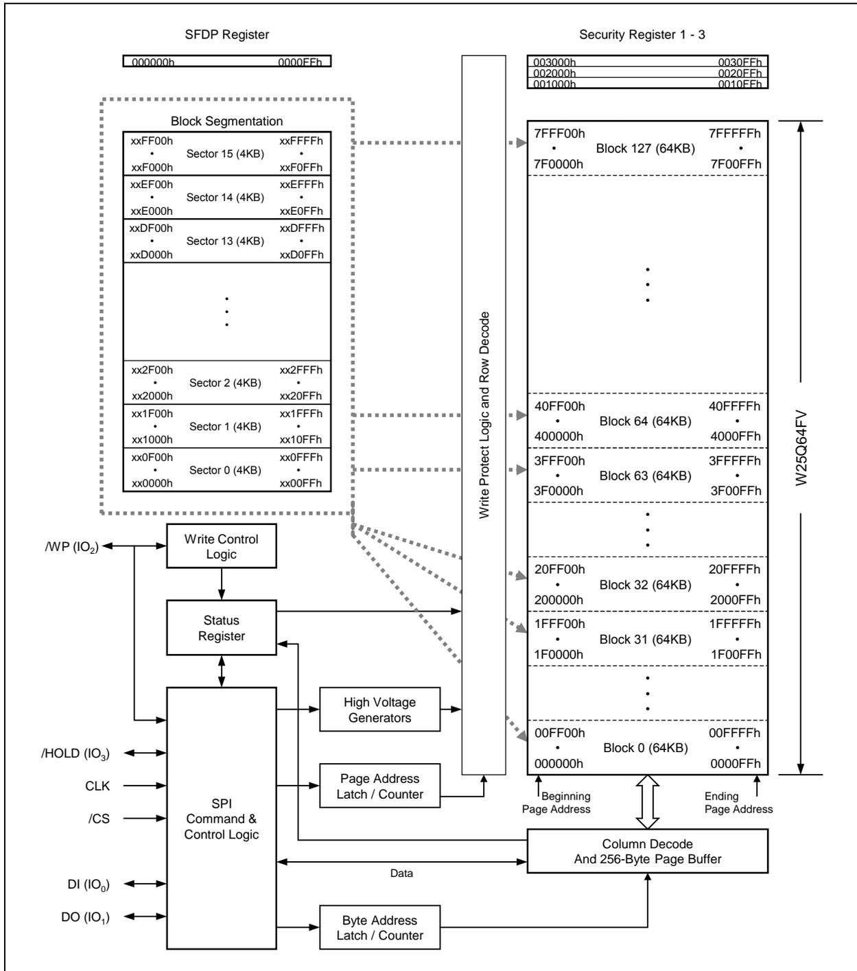
Figure 2. W25Q64FV Serial Flash Memory Block Diagram
