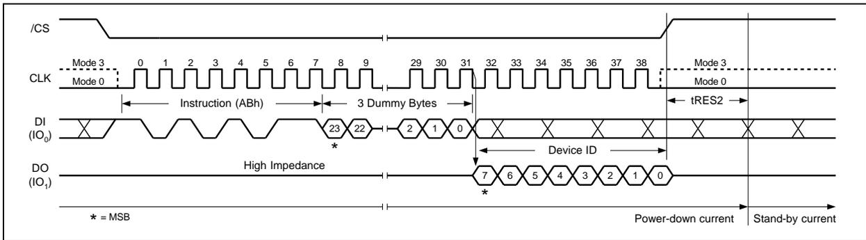
Figure 28c. Release Power-down / Device ID Instruction (SPI Mode)
