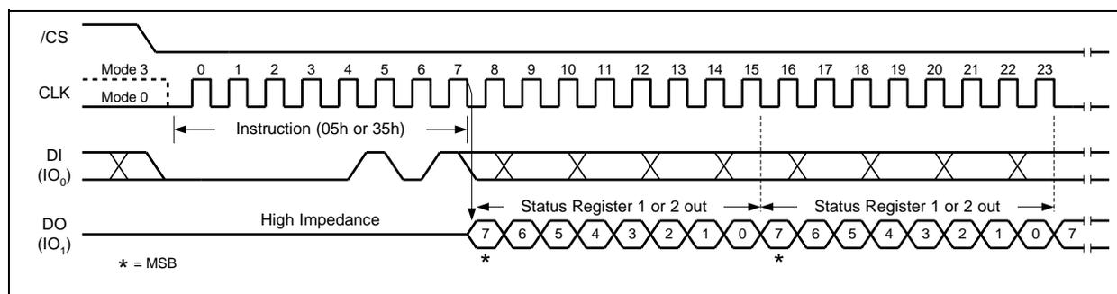
Figure 8a. Read Status Register Instruction (SPI Mode)
