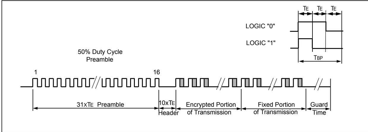
**FIGURE 9-4: PWM PREAMBLE/HEADER FORMAT (MOD=0)**
