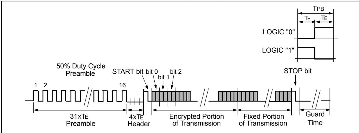
**FIGURE 9-7: MANCHESTER PREAMBLE/HEADER FORMAT (MOD=1)**
