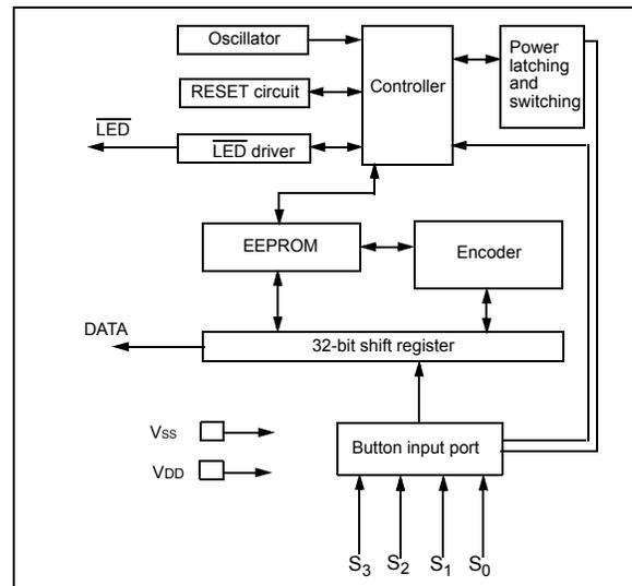
The HCS360 combines a 32-bit hopping code generated by a nonlinear encryption algorithm, with a 28/32-bit serial number and 7/3 status bits to create a 67-bit transmission stream.
