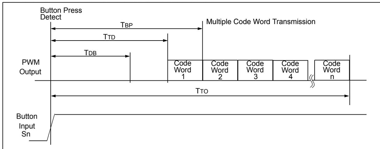
**FIGURE 9-2: POWER-UP AND TRANSMIT TIMING REQUIREMENTS**
