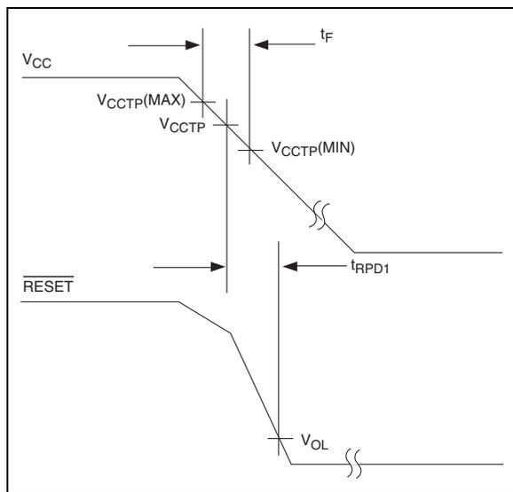
**FIGURE 3-2:** Timing Diagram – Power Down (TC1275/TC1276).
