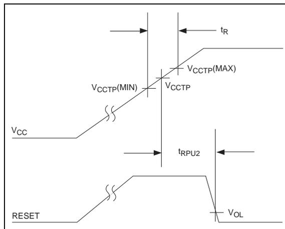
**FIGURE 3-3:** Timing Diagram – Power Up (TC1277).
