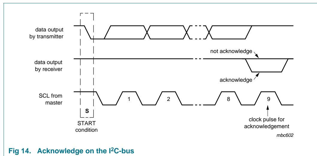
**Fig 14. Acknowledge on the I<sup>2</sup>C-bus**
