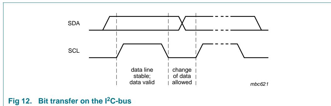
**Fig 12. Bit transfer on the I<sup>2</sup>C-bus**
