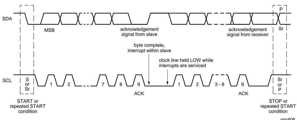
**Fig 15. Data transfer on the I<sup>2</sup>C-bus**
