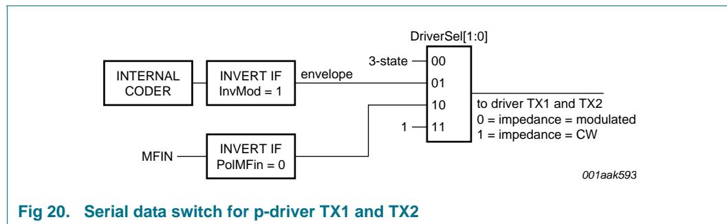
Fig 20. Serial data switch for p-driver TX1 and TX2
