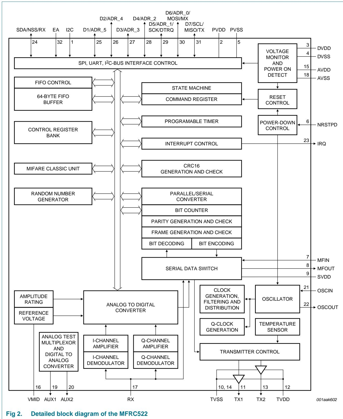
Fig 2. Detailed block diagram of the MFRC522
