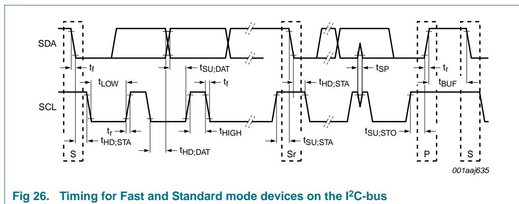
Fig 26. Timing for Fast and Standard mode devices on the I<sup>2</sup>C-bus
