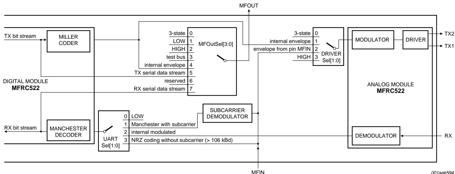
Fig 21. Overview of MFIN and MFOUT signal routing
