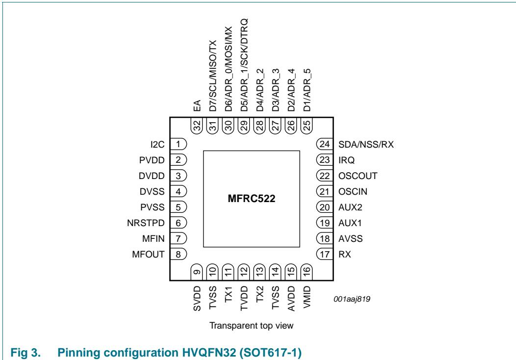
**Fig 3. Pinning configuration HVQFN32 (SOT617-1)**
