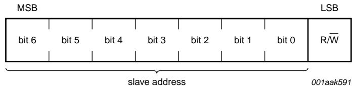
**Fig 16. First byte following the START procedure**
