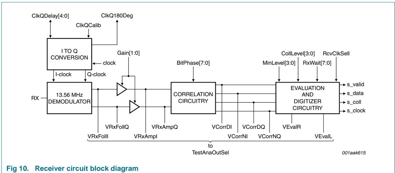
Fig 10. Receiver circuit block diagram
