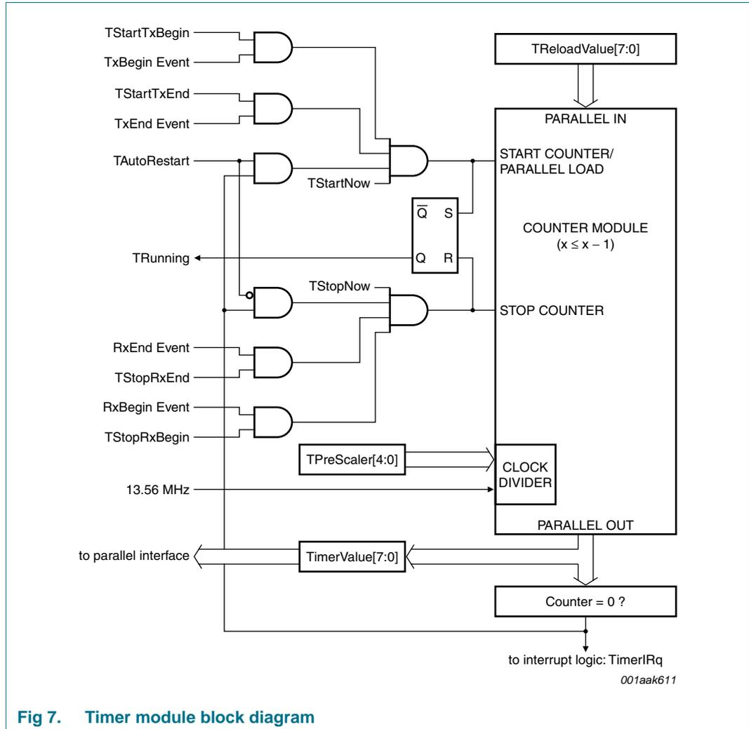
Fig 7. Timer module block diagram
