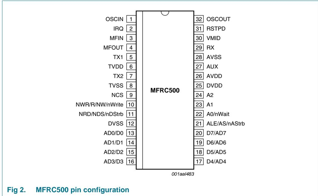
Fig 2. MFRC500 pin configuration
