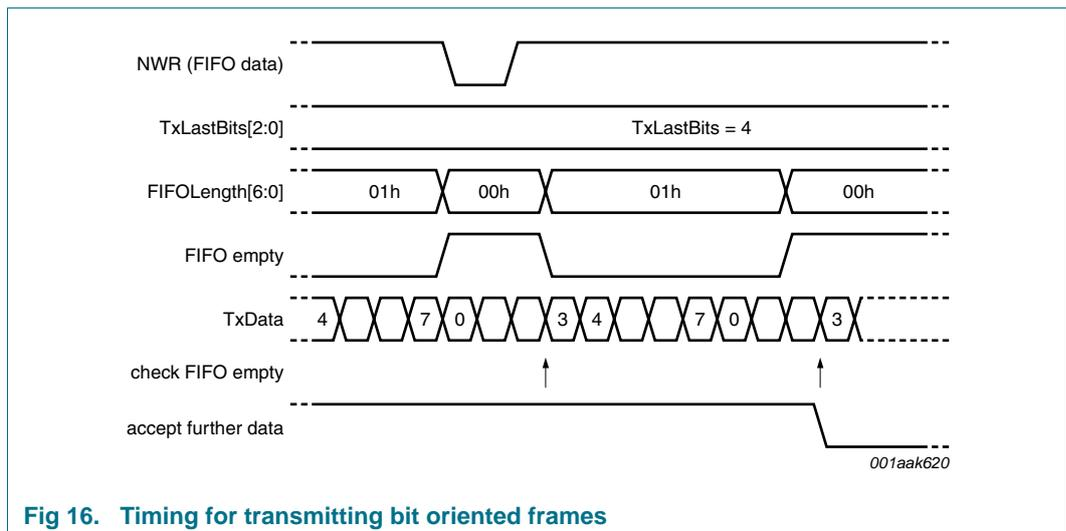
Fig 16. Timing for transmitting bit oriented frames
