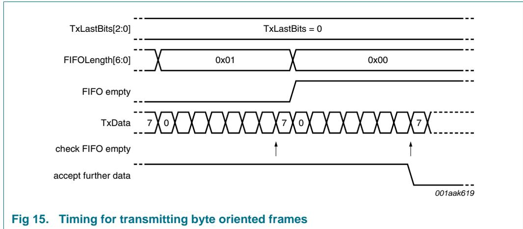
Fig 15. Timing for transmitting byte oriented frames
