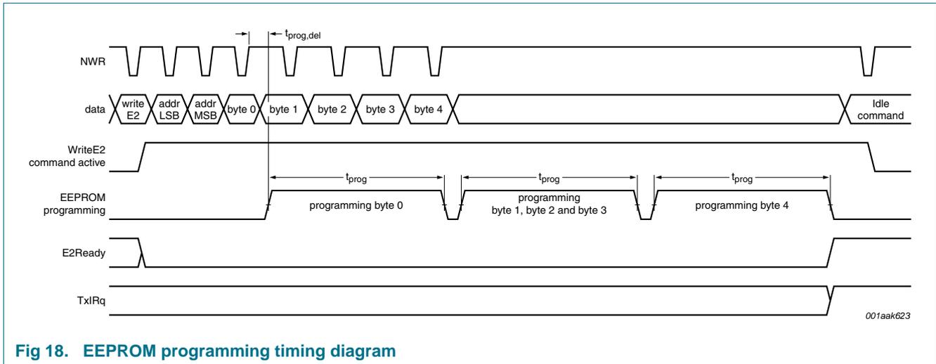
Fig 18. EEPROM programming timing diagram
