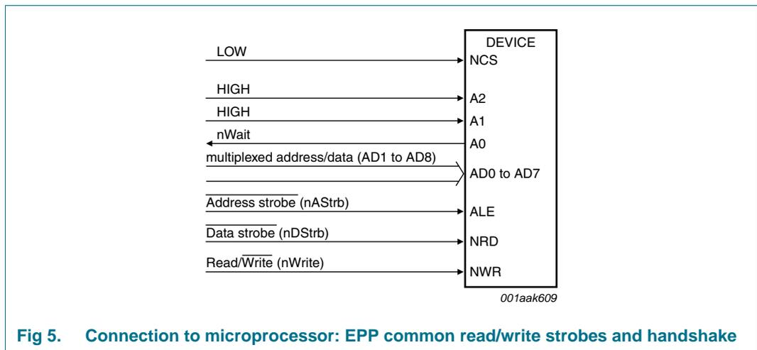
Fig 5. Connection to microprocessor: EPP common read/write strobes and handshake
