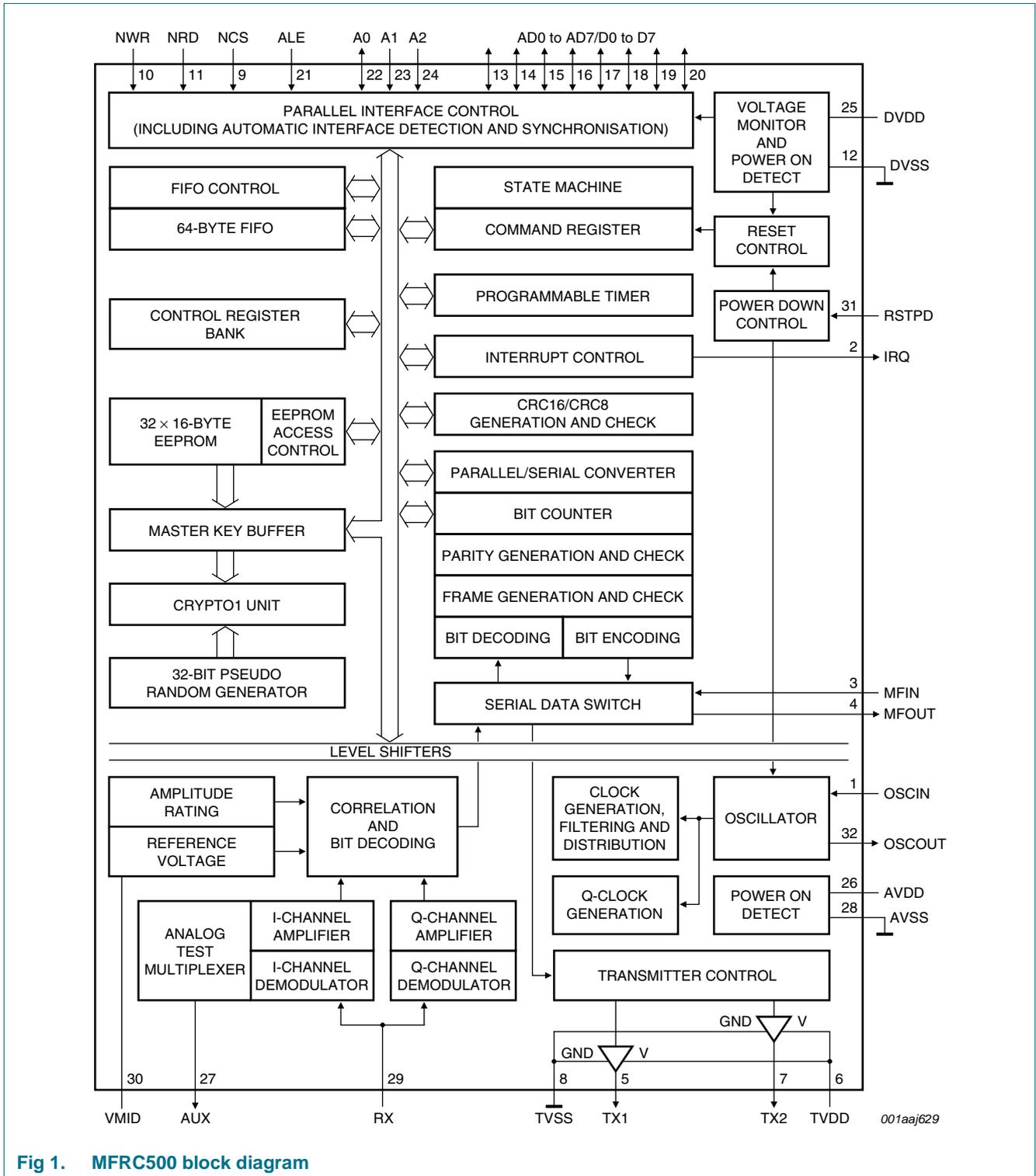
Fig 1. MFRC500 block diagram
