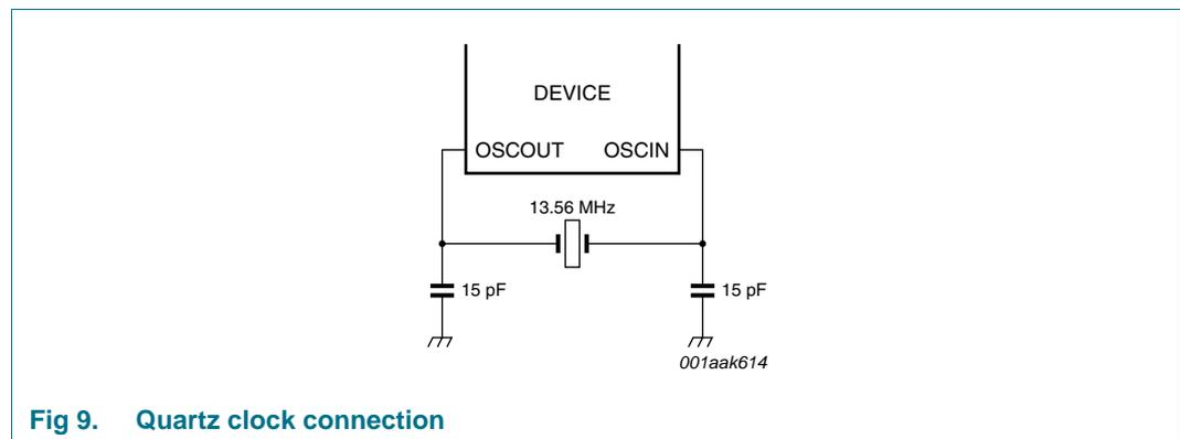
The clock applied to the MFRC500 acts as a time basis for the synchronous system encoder and decoder. The stability of the clock frequency is an important factor for correct operation. To obtain highest performance, clock jitter must be as small as possible. This is best achieved by using the internal oscillator buffer with the recommended circuitry.
