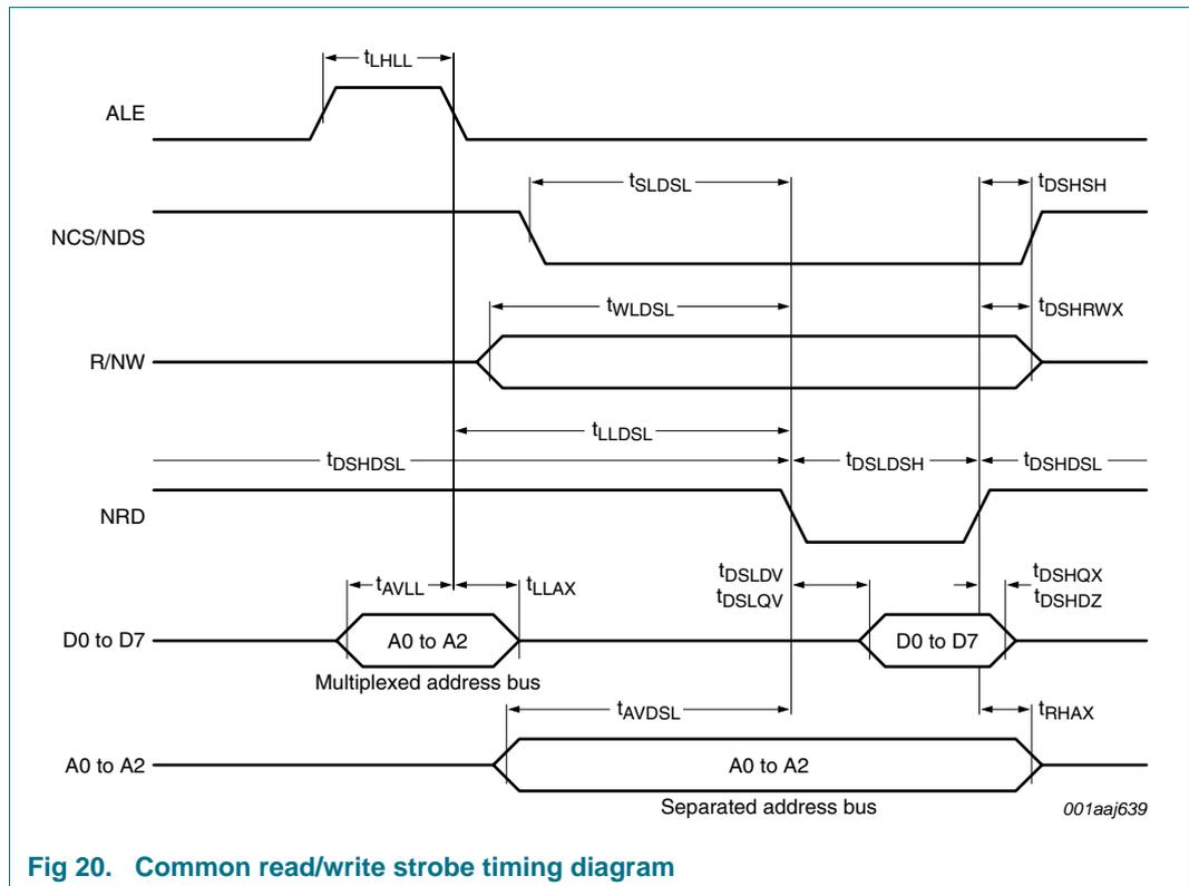
Fig 20. Common read/write strobe timing diagram
