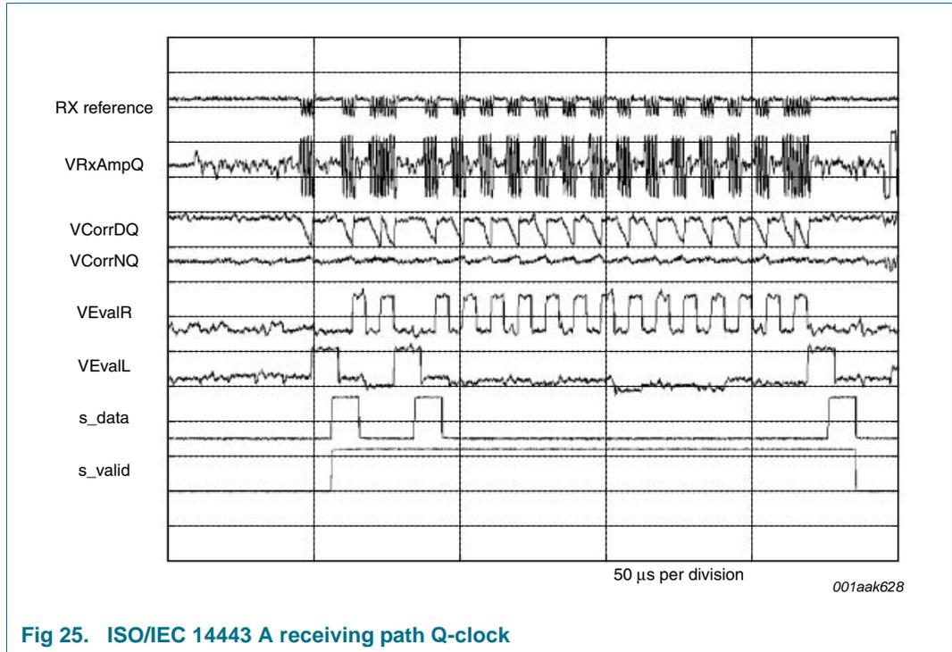
**Fig 25. ISO/IEC 14443 A receiving path Q-clock**
