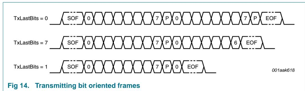
**Fig 14. Transmitting bit oriented frames**
