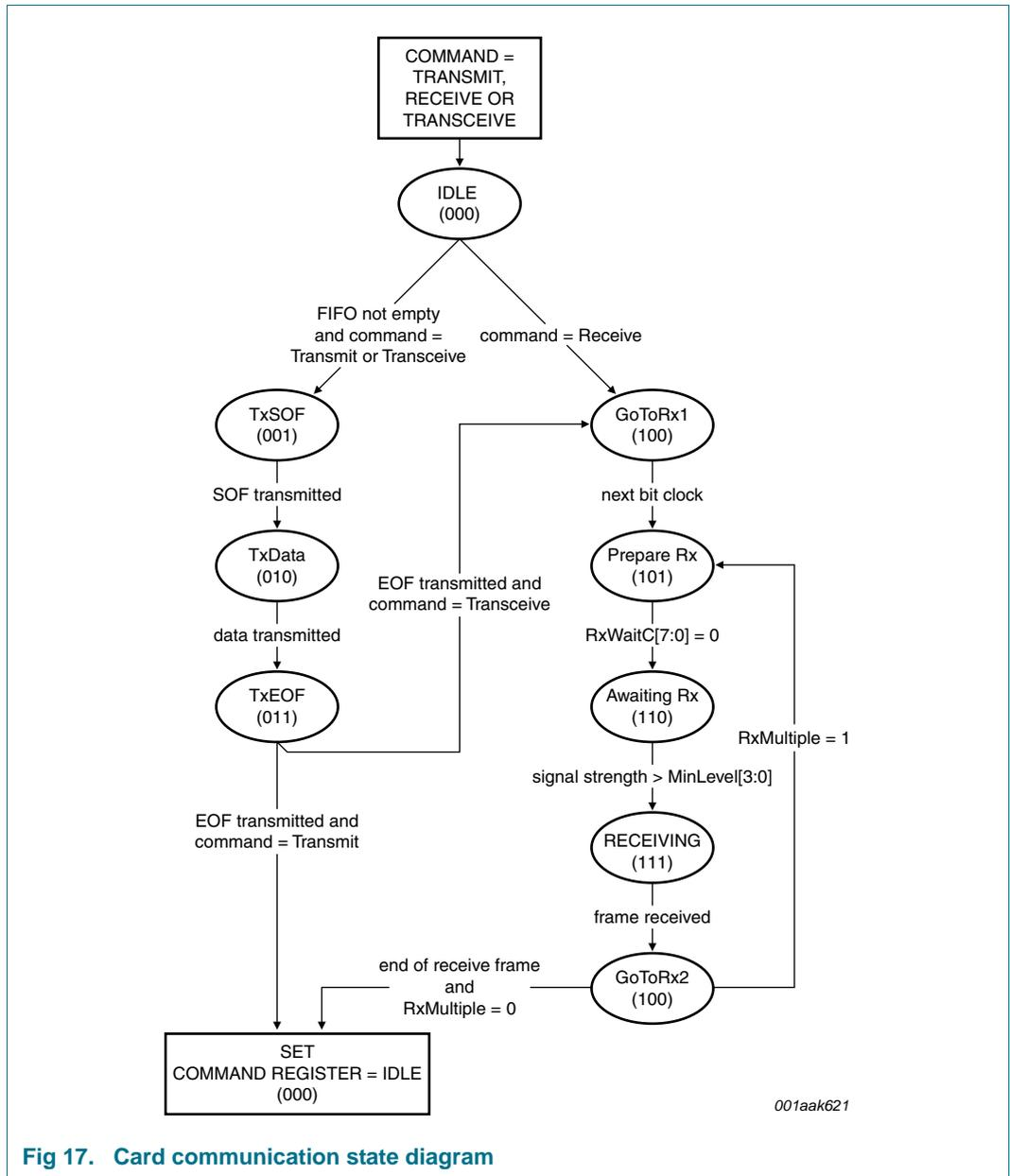
Fig 17. Card communication state diagram
