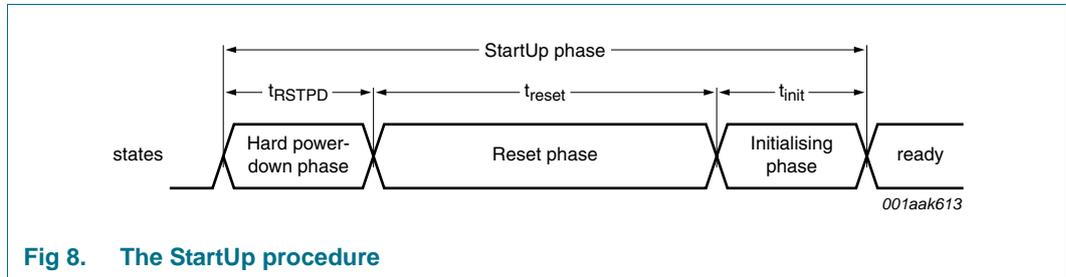
Fig 8. The StartUp procedure
