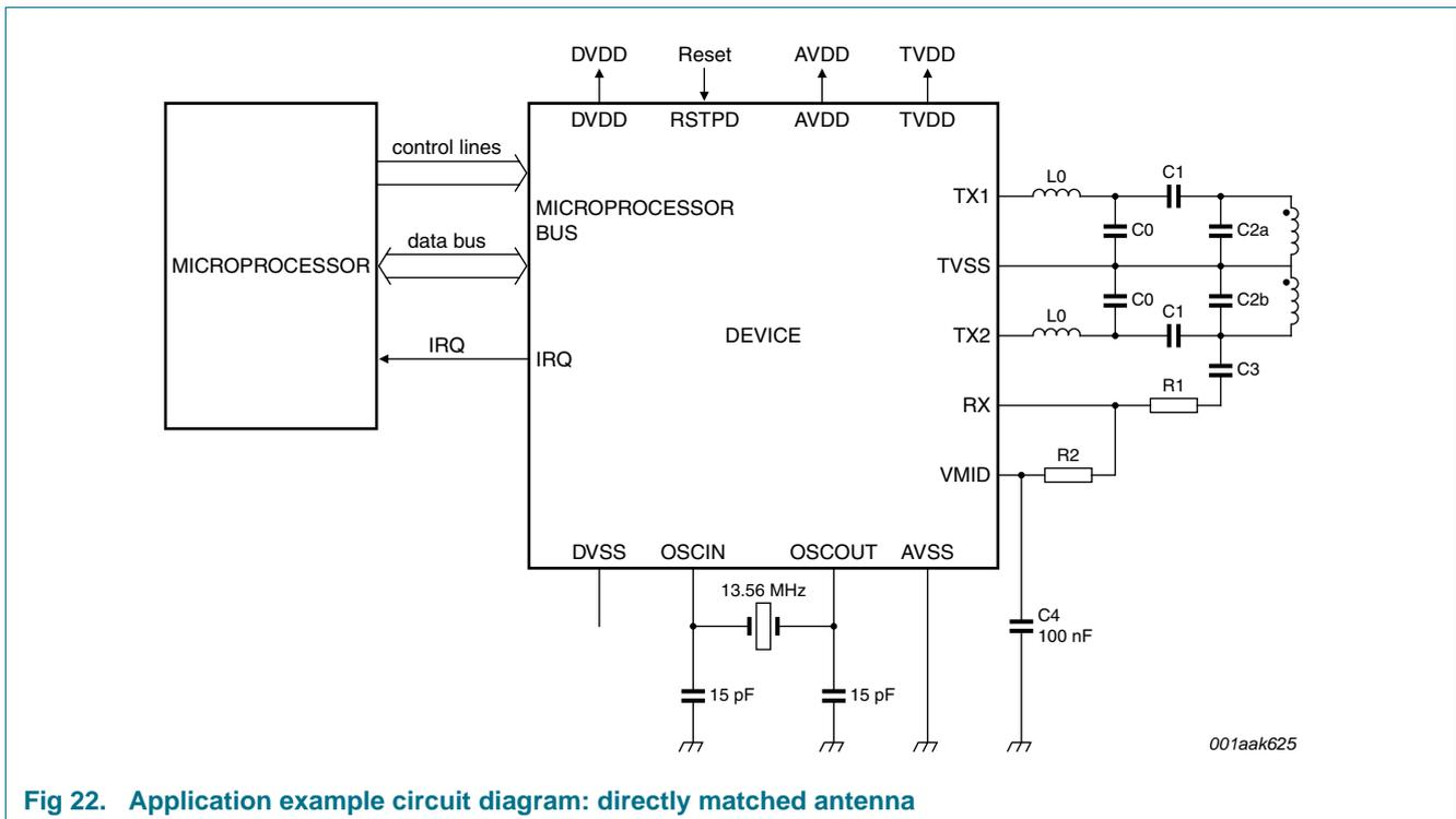
Fig 22. Application example circuit diagram: directly matched antenna
