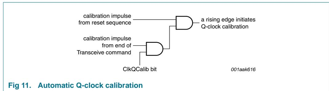
**Fig 11. Automatic Q-clock calibration**
