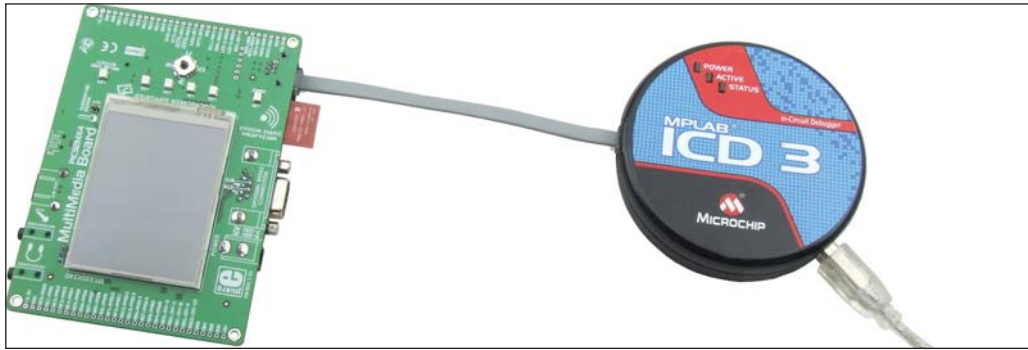
Figure 16-1: MultiMedia Board connected to ICD3 programmer
