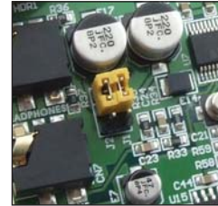
Figure 14-3: Jumpers J1 and J2 in upper position
