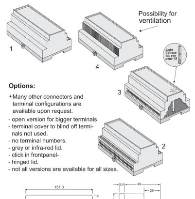
Module enclosure for M36 DIN-rail. Series 1570 is, if requested, available in several colours and with customer specified holes in the front.
