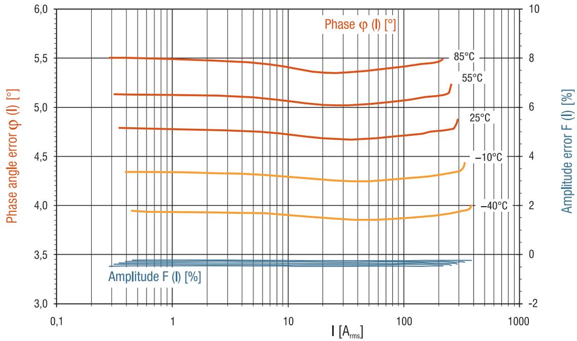
Fig. 6: 120 A with DC Tolerance, T60404-E4627-X101
