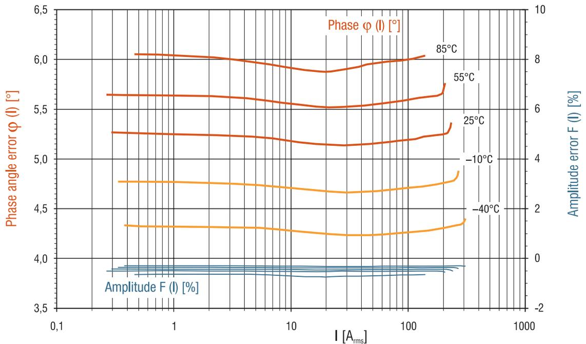
Fig. 5: 100 A with DC Tolerance, T60404-E4626-X101/-X501/-X151
