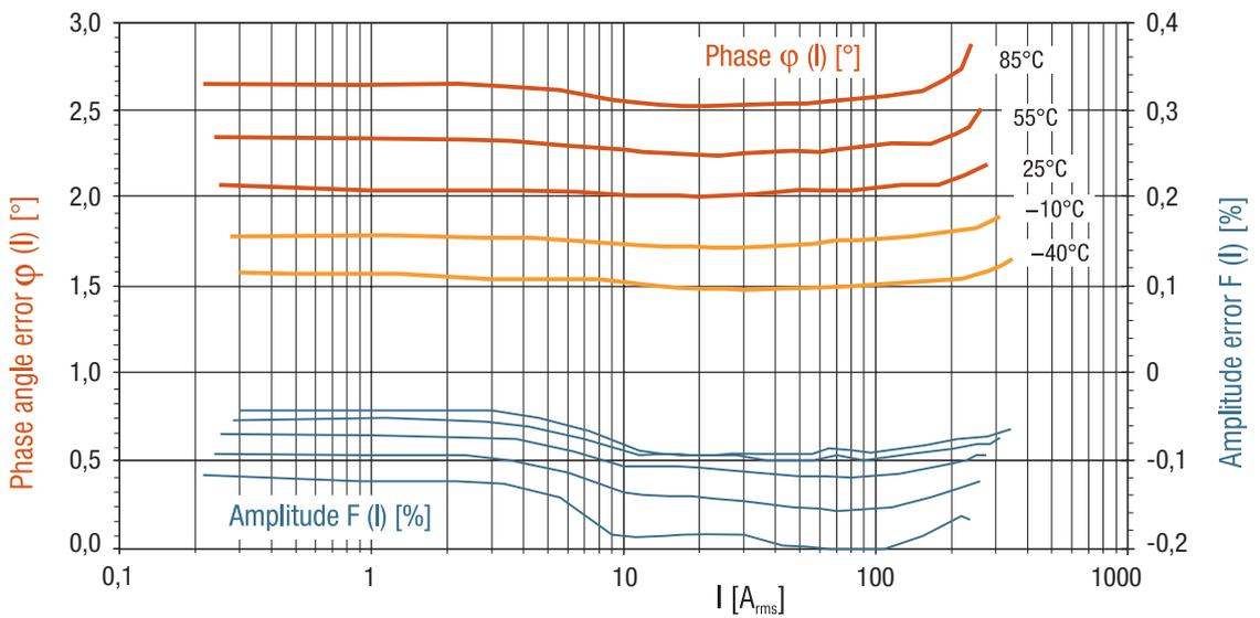
Fig. 9: 60 A with DC Tolerance, T60404-E4624-X121/-X171
