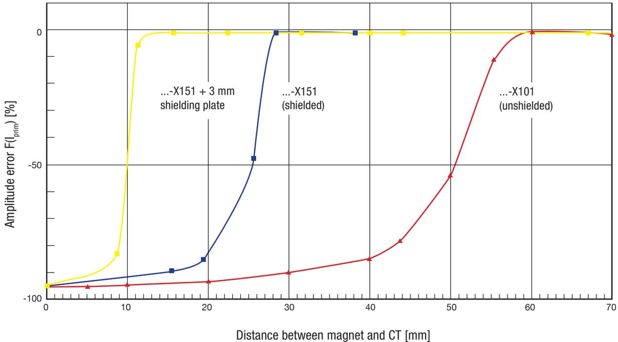
Diagram above shows a comparison of different shielding configurations. For optimum protection against external magnetic fields CTs from ...-X151 series and a 3 mm shielding plate are needed.
