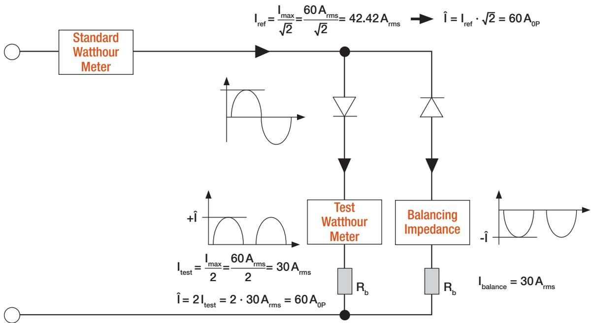
The diagram above shows a typical test of DC tolerance of a 60 A electricity meter. The Balancing Impedance is another meter from the same series. During this test, the meter shows 30 A<sub>rms</sub>, which is equal to 60 A<sub>0P</sub> for only half-rectified sinusoidal currents.
