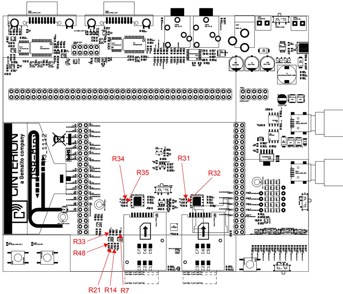
Figure 9: Placement, Page 2 (with Starter Kit mounted)
