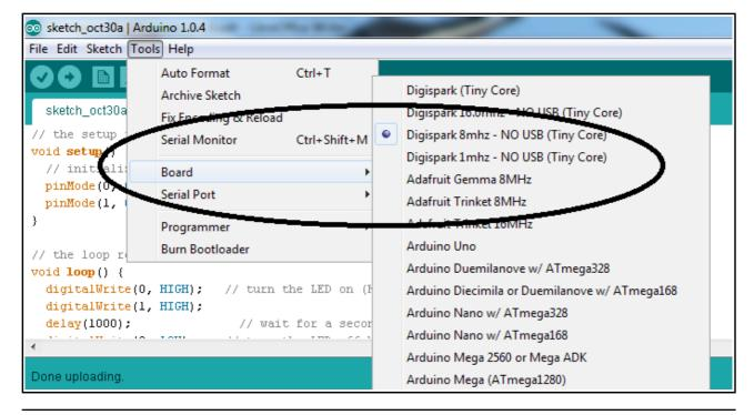
OLIMEXINO-85 is recognized as "Digispark 8mhz - NO USB (Tiny Core)" under "Tools → board"
