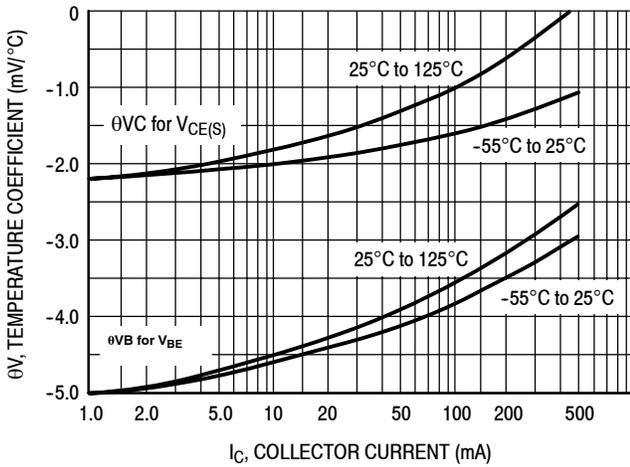
Figure 3. Temperature Coefficients
