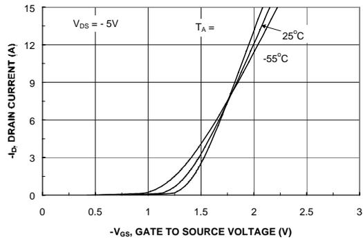
Figure 5. Transfer Characteristics.
