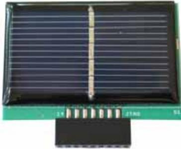
**MSP430-SOLAR** is power supply module with solar panel and re-chargeable battery. The solar panel is rated 2.4V 80mA and have on board DC/DC voltage boost converter which generates 3.3V for the MSP430 target.
