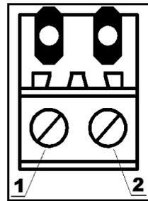
This connector is used to power the MOD-GSM-EDGE. External (+9-12VDC) power source have to be applied to this pins.
