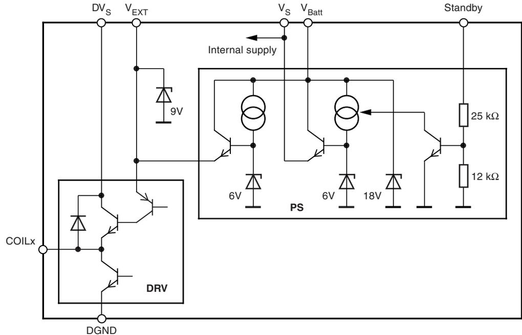
The U2270B can be operated with one external supply voltage or with two externally-stabilized supply voltages for an extended driver output voltage or from the 12V battery voltage of a vehicle. The 12V supply capability is achieved via the on-chip power supply (see [Figure 3-1](#)). The power supply provides two different output voltages,  $V_S$  and  $V_{EXT}$ .
