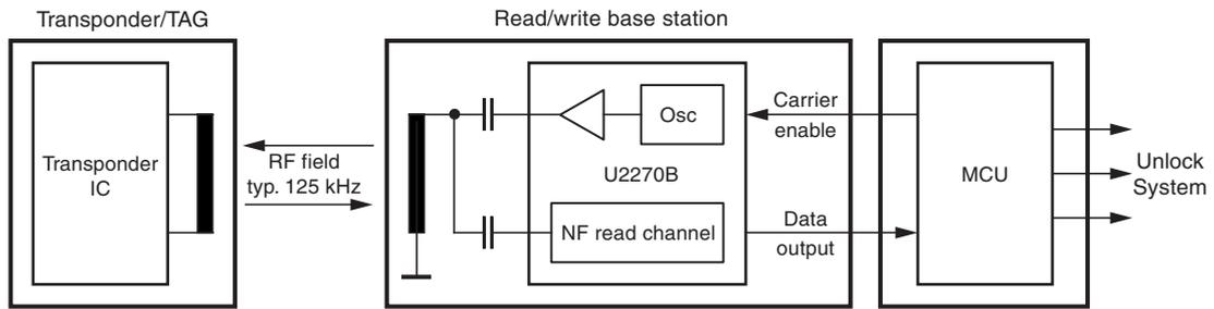
**Figure 1-2.** Block Diagram
