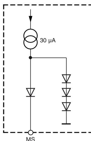
**Figure 3-10.** Equivalent Circuit of Pin CFE
