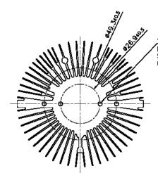
4-#2.8±0.3, depth:5mm For LED Module Assembly Screw torque max 12kgf.cm Using M3 Tapping Screw
