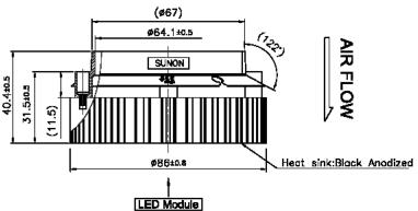
Assembly direction of customer's LED Module
