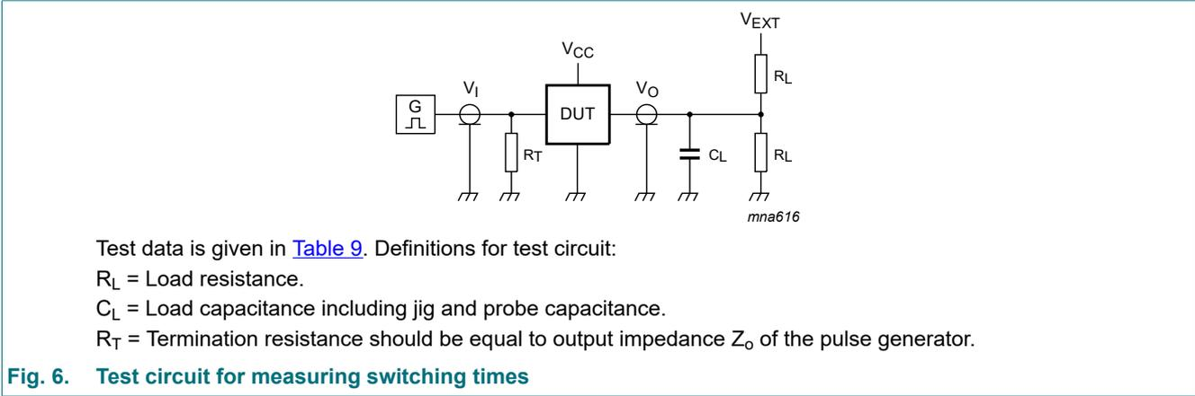
**Fig. 6. Test circuit for measuring switching times**
