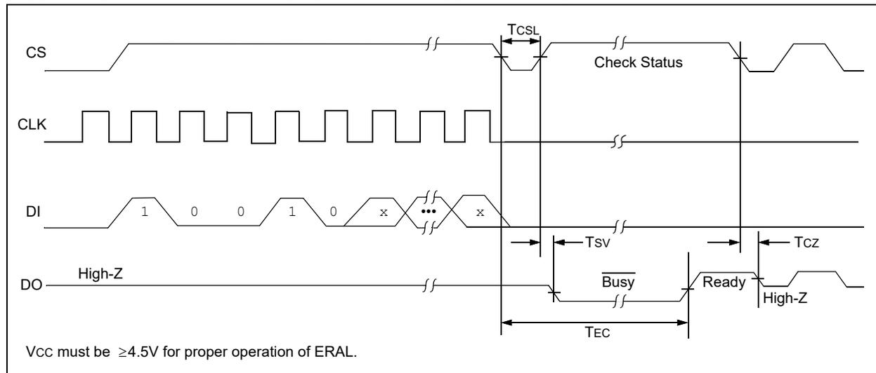
**FIGURE 2-4: ERAL TIMING FOR 93C DEVICES**
