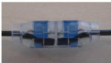
Wires terminated correctly
