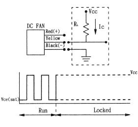
Vcc = FAN Vcc Ic = 5mA MAX Ic=VCC/RL
