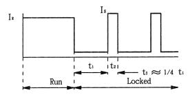
3rd wire signal Run : Square Wave Locked : V#
