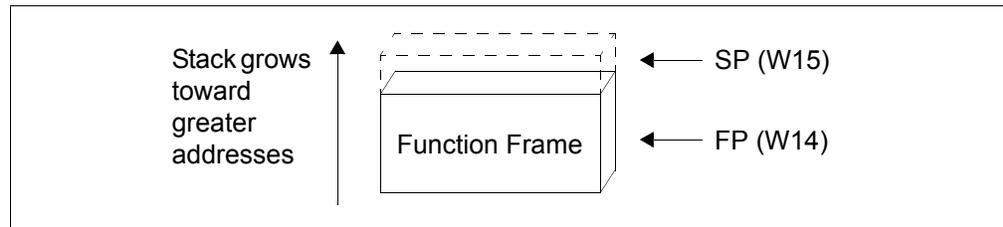
The C run-time startup modules in `libpic30-omf.a` initialize the Stack Pointer W15 to point to the bottom of the stack and initialize the Stack Pointer Limit register to point to the top of the stack. The stack grows up and if it should grow beyond the value in the Stack Pointer Limit register, then a stack error trap will be taken. The user may initialize the Stack Pointer Limit register to further restrict stack growth.
