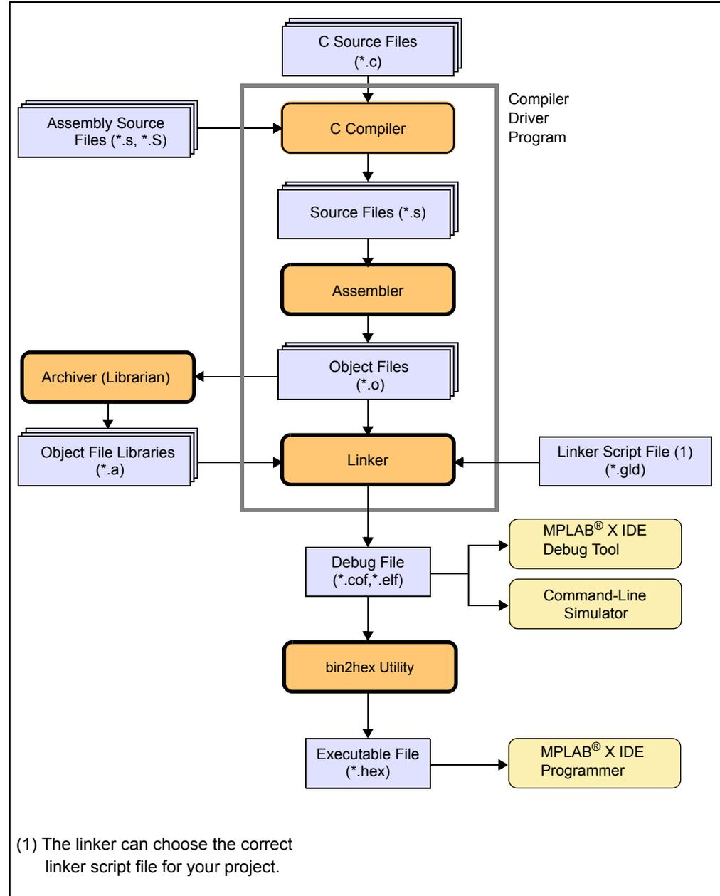
In this MPLAB X IDE project, C source files are shown as input to the compiler. The compiler will generate source files for input into the assembler. For more information on the compiler, see the compiler documentation.
