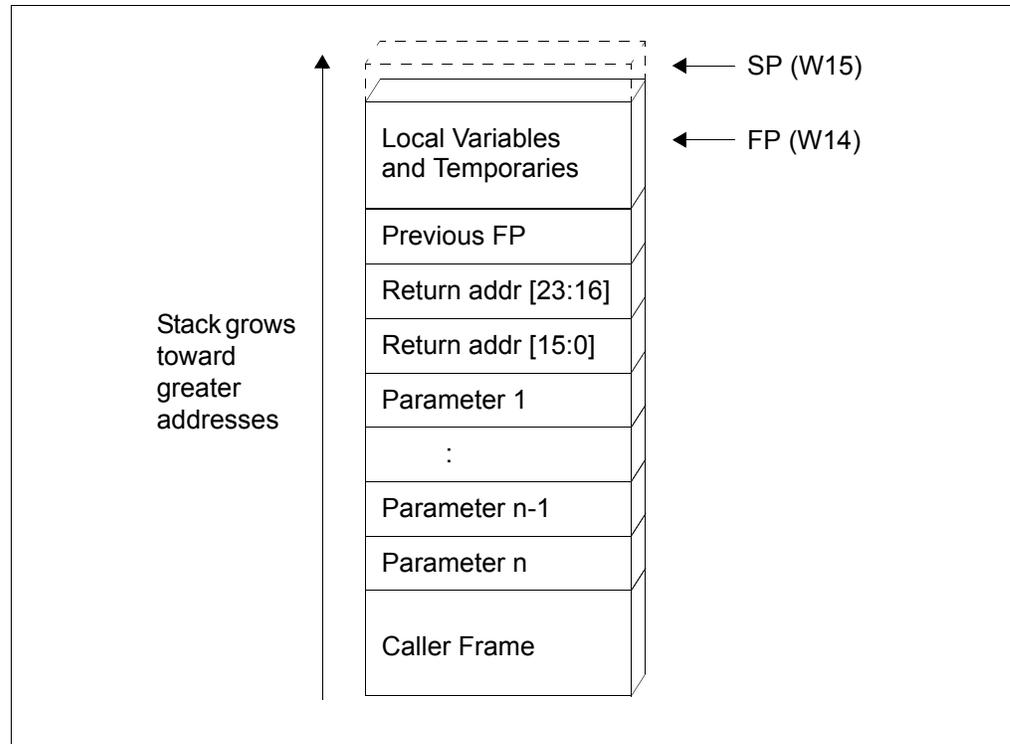
Finally, any callee-saved registers that are used in the function are pushed (Figure 10-4).
