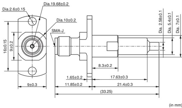
Measurement Probe for MM8030-2610
