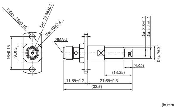
Measurement Probe for MM8130-2600/MM8430-2610
