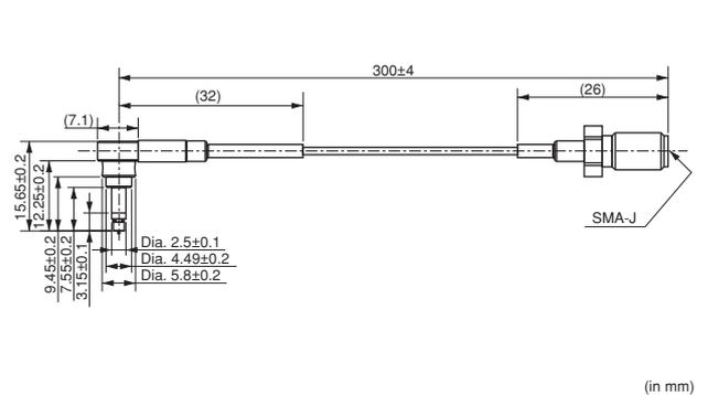
Measurement Probe for MM8130-2600/MM8430-2610
