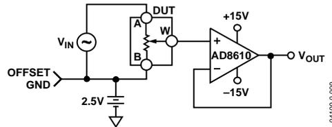
Figure 34. Test Circuit for Gain vs. Frequency
