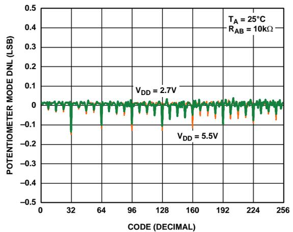
Figure 11. DNL vs. Code vs. Supply Voltages
