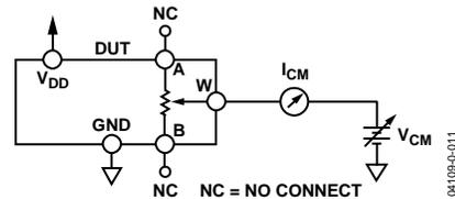
Figure 36. Test Circuit for Common-Mode Leakage Current
