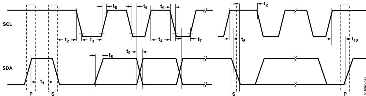
Figure 3. I<sup>2</sup>C Interface Detailed Timing Diagram
