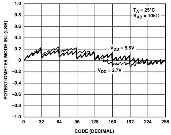
Figure 10. INL vs. Code vs. Supply Voltages
