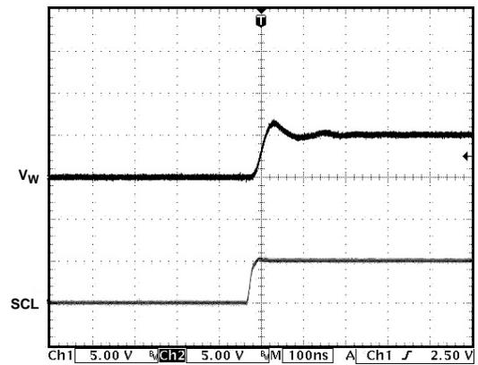
Figure 29. Large-Signal Settling Time
