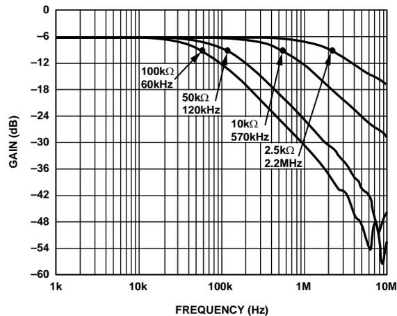
Figure 23.  $-3\text{ dB}$  Bandwidth at Code = 0x80
