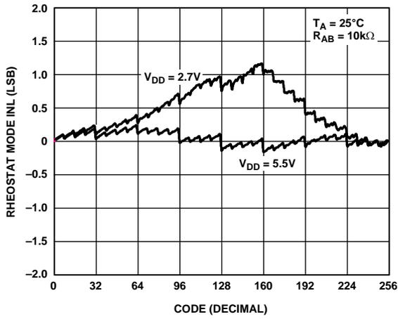
Figure 6. R-INL vs. Code vs. Supply Voltages
