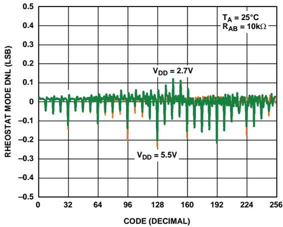
Figure 7. R-DNL vs. Code vs. Supply Voltages
