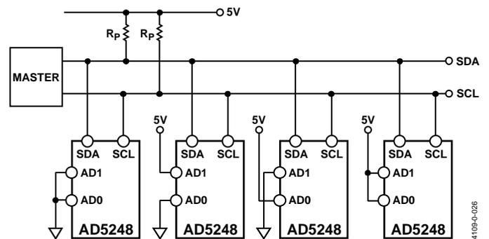
Figure 49. Multiple AD5248 Devices on One I<sup>2</sup>C Bus
