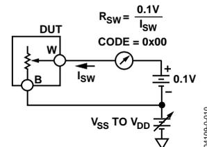
Figure 35. Test Circuit for Incremental On Resistance
