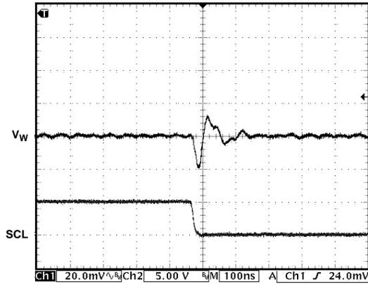
Figure 25. Digital Feedthrough
