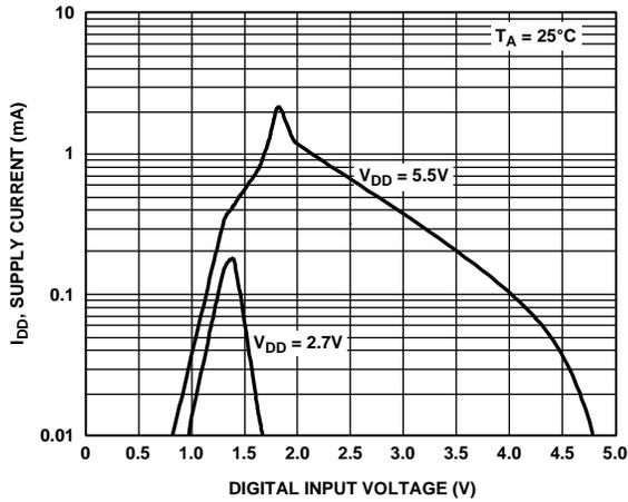
Figure 24. Supply Current vs. Digital Input Voltage
