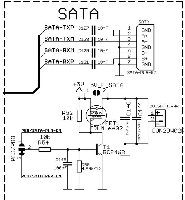
There is a 5V\_SATA\_PWR connector that is suitable for powering 5V hard-disks through the board. To keep the low form factor we have placed the small JST connector.
