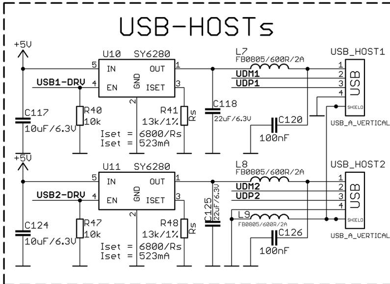
There are two USB host connector featured on the board. They are called USB\_HOST1 and USB\_HOST2. Each of them has own connector, both situated near the Ethernet connector. Each of connector has own low loss power distribution switch SY6280 which protects the board in case the devices you have plugged to the board try to draw more current than 523mA combined. The maximum current available on each of the USB hosts is exactly 523mA.
