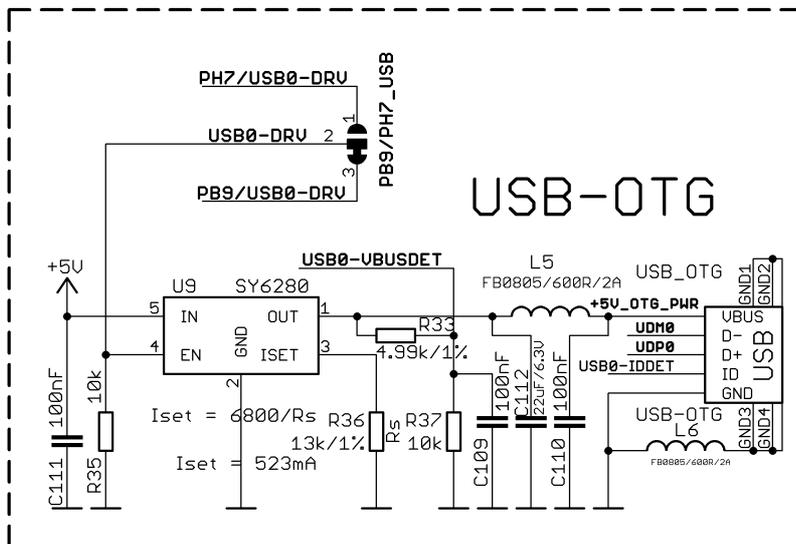
The USB\_OTG features Low Loss Power Distribution Switch SY6280 which protects the board in case the devices you have plugged to the USB\_OTG attempt to draw more current than 523mA combined. The maximum current available on the 5V USB\_OTG is exactly 523mA.
