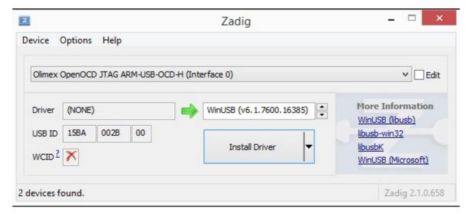
If Zadig doesn't do the job or you are using OpenOCD version prior to 0.8.0 the more robust method is to download an archive with the drivers and point the Windows Device Manager to it manually. Links to those resources might be found at the end of this chapter!
