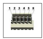
**PGED2** conducts I/O operations for the "Program Data" signal. Serial data for programming. **PGEC2** serves only as input for the "Program Clock" signal. Clock used for transferring the serial data (output from ICSP, input for the MCU).
